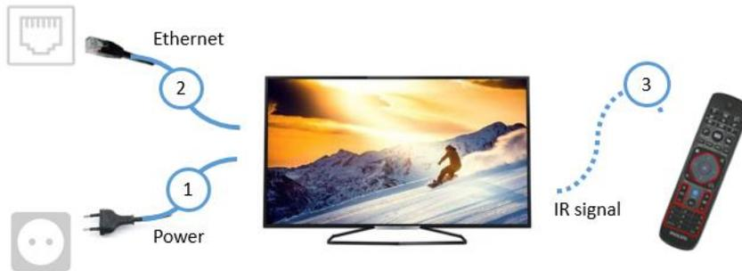
1. Power supply port DC 12V out, max 1,5A (to wall power outlet).
